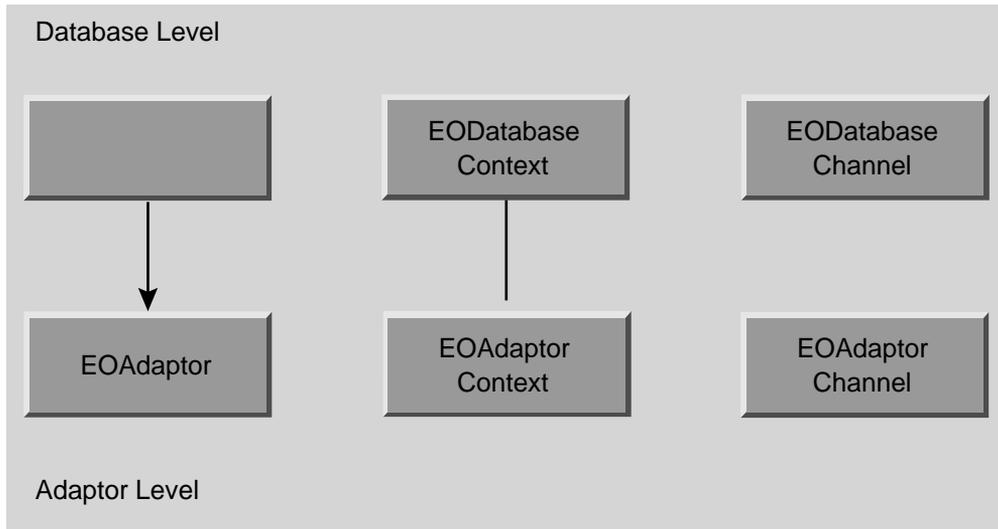
The database level acts as an intermediary between the adaptor level and the **control layer** , which includes an EObjectStoreCoordinator and an EOEditingContext (Figure 0-2). The control layer operates in terms of enterprise objects, while the adaptor level operates in terms of database rows packaged as NSDictionary. It's the job of the database level to perform the necessary object-to-relational translation between the two.
